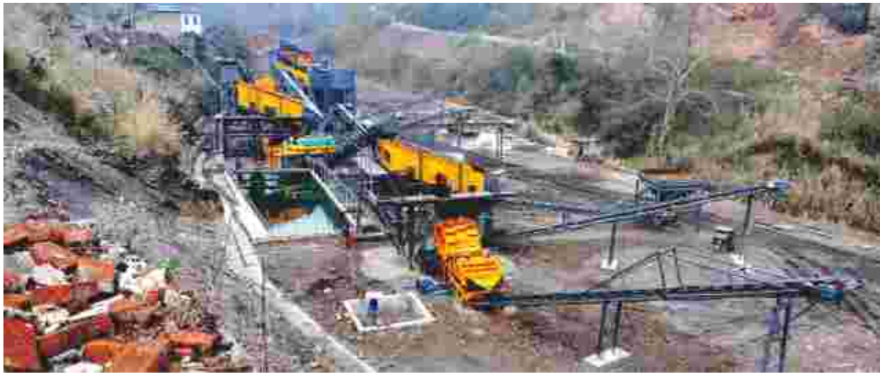
宜都时产300吨洞渣尾矿处理生产线 Yidu Time produces 300 tons per hour of mining waste treatment line
