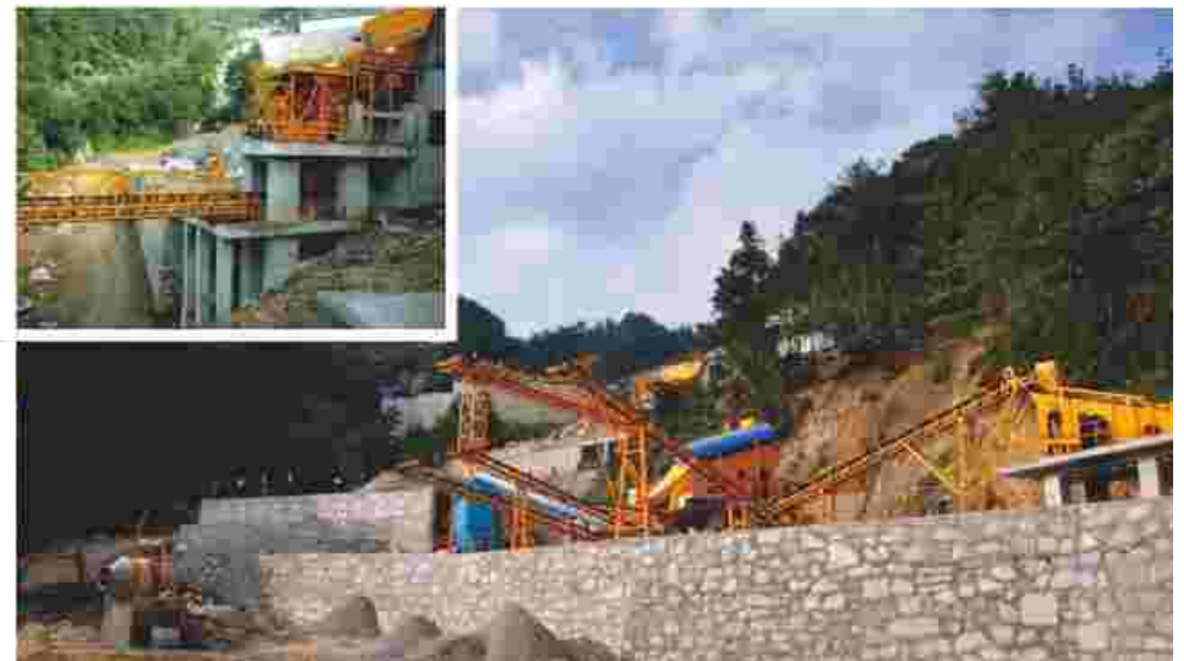
宜昌时产500吨花岗岩破碎生产线 Yichang-time 500 tons per hour of granite crushing line
