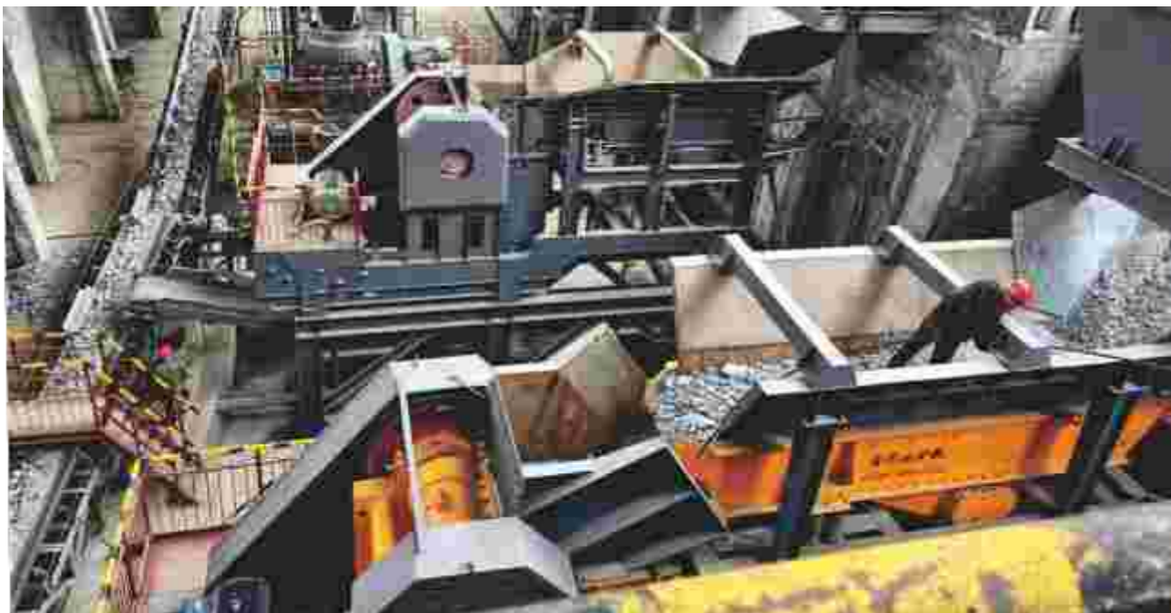
化工集团时产500吨磷矿石破碎生产线 Chemical group produces 500 tons per hour of phosphate ore crushing line
